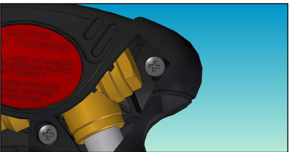
Centraggi corpo su scocche Corpo pistola in ottone stampato Valve body centered on the shells for a perfect matching and greater strength of the gun. Gun valve body in forged brass
